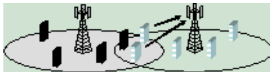
Figure h61—Relaying of the ADV-REQ message MATIs content by the slave SSs to their home system
