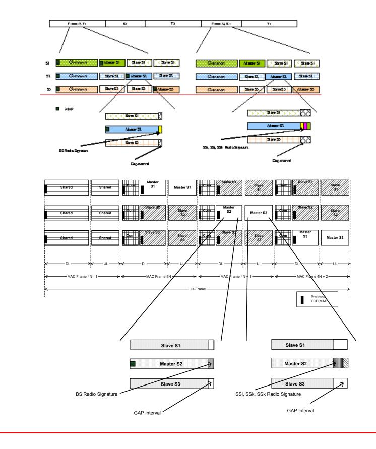
Figure h51—Allocation of slots for BS and SS radio signature
