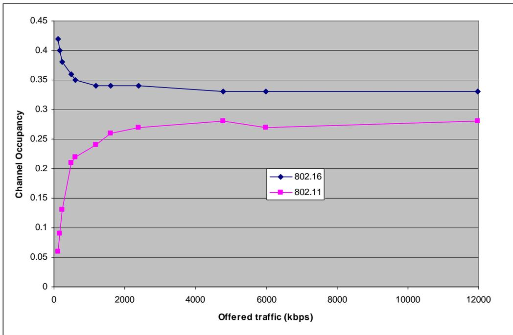
**Figure 6** Collocated simulation configuration – considering fair sharing for 2 802.16 Systems at channel capacity (offered load at 1.5Mbps per link) and 1 802.11 System with varying offered load. UtilizationGoal=100% (i.e. not set)
