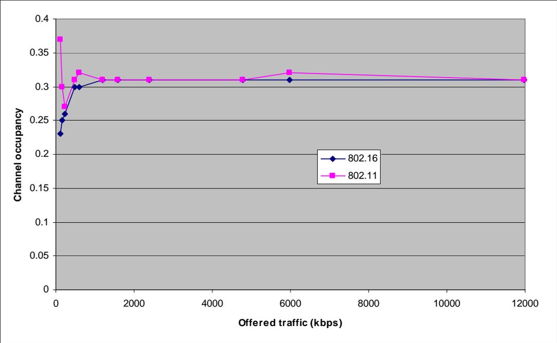
**Figure 9** Collocated simulation configuration – considering fair sharing for 1 802.11 System at channel capacity (offered load at 1.5Mbps per link) and 2 802.16 Systems with varying offered load. UtilizationGoal=33%.
