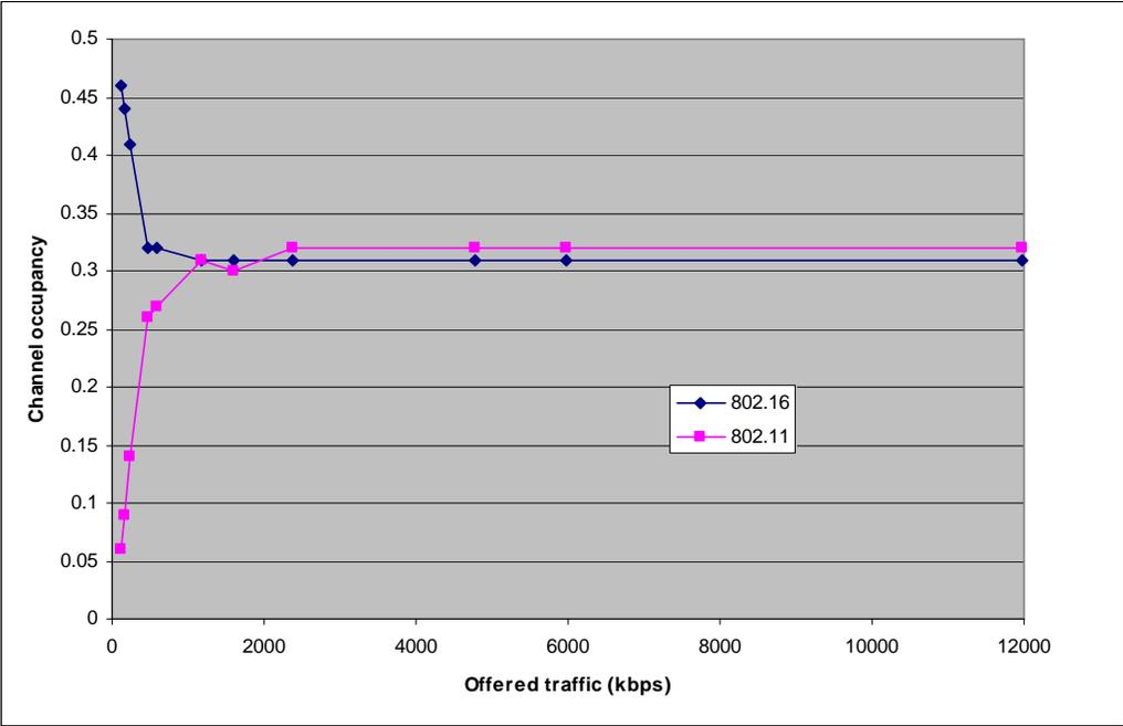
**Figure 7** Collocated simulation configuration – considering fair sharing for 2 802.16 Systems at channel capacity (offered load at 1.5Mbps per link) and 1 802.11 System with varying offered load. UtilizationGoal=33%.
