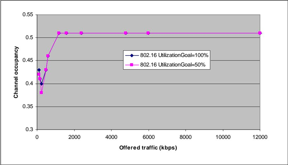
**Figure 3** Collocated simulation configuration – demonstrating fair sharing for 2 802.16 systems. *UtilizationGoal=100%* (i.e. not set).
