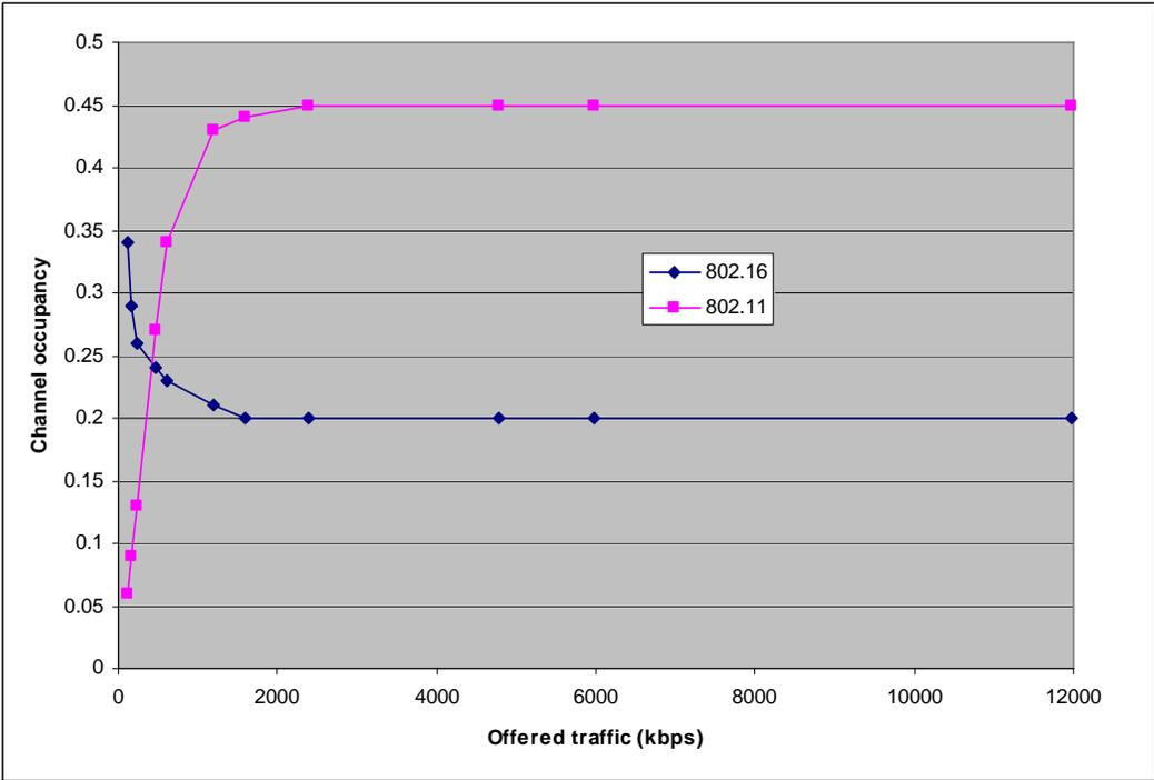
**Figure 11** Collocated simulation configuration – considering fair sharing for 2 802.16 Systems and 1 802.11 System. UtilizationGoal=33%. 47 symbols per frame, downlink=28, uplink=19.
