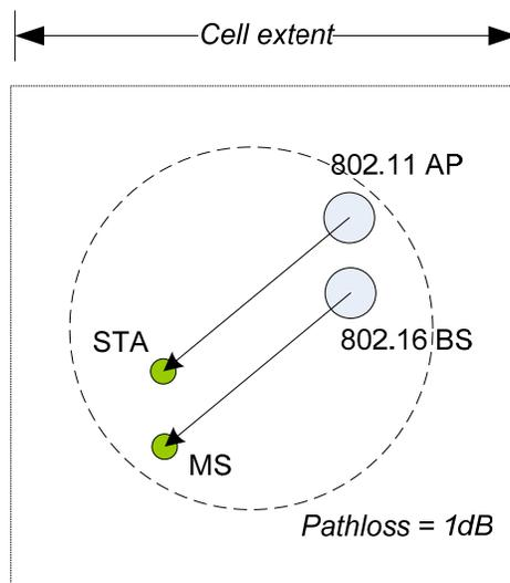
**Figure 2** Collocated simulation configuration.
