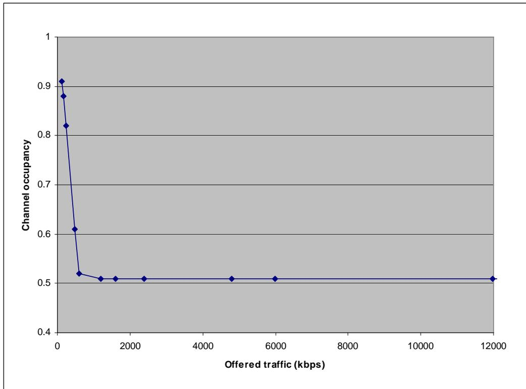
**Figure 13** 1 802.16 Systems. *UtilizationGoal=100%*. 47 symbols per frame, downlink=28, uplink=19. For the case of 46 symbols per frame, downlink=28, uplink=18 channel occupancy is 100% for all offered traffic.
