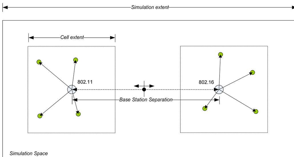
**Figure 14** Collocated simulation configuration: 1 802.16 system and 1 802.11 system.
