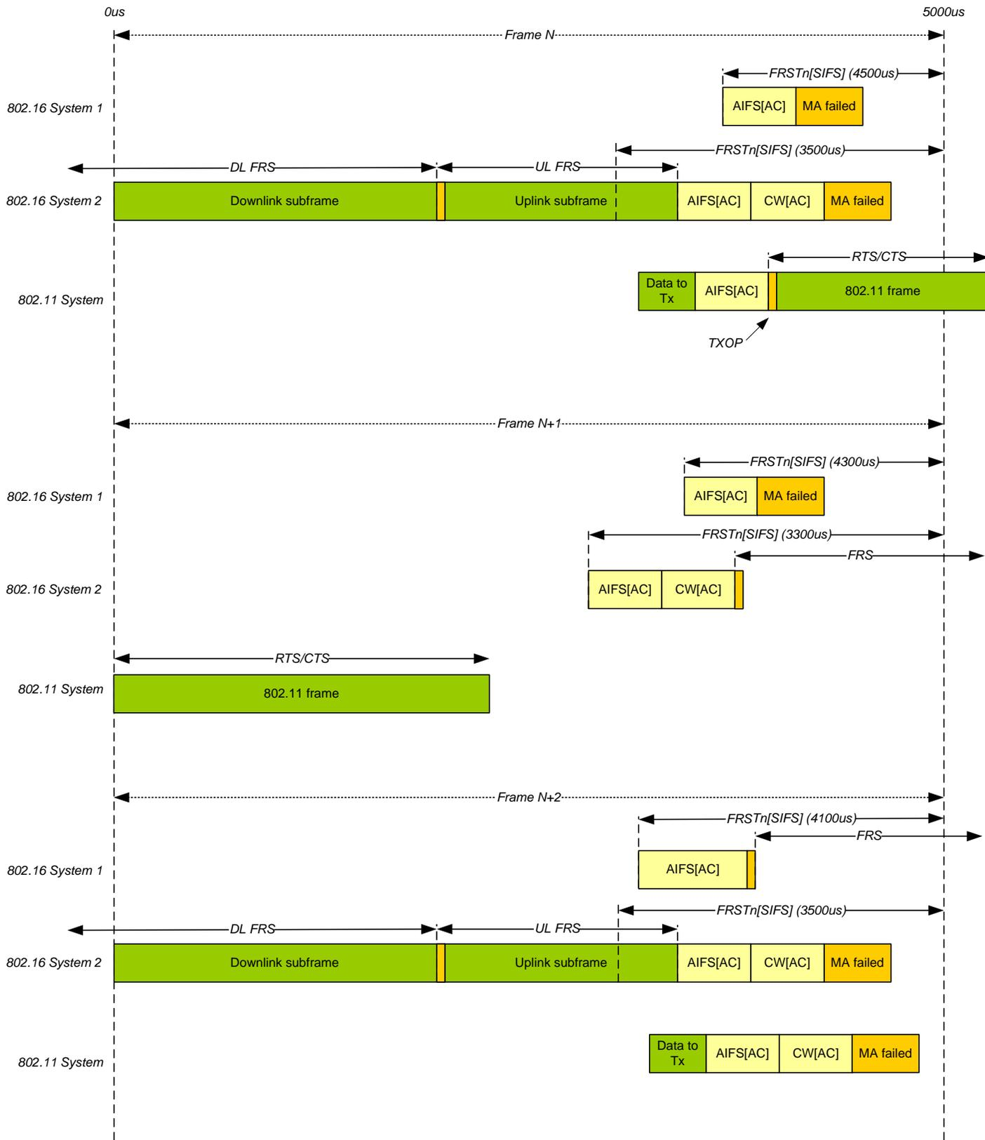
**Figure 1** A detailed example of 2 802.16 and 1 802.11 systems sharing the medium over 3 frame intervals. 802.16 System 2 has Frame N, 802.11 uses Frame N+1, and 802.16 System 2 claims Frame N+2. 802.16 System 1 claims Frame N+3.
