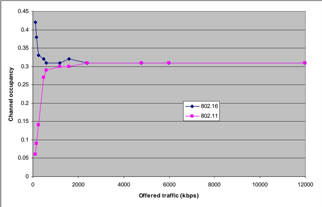
**Figure 10** Collocated simulation configuration – considering fair sharing for 2 802.16 Systems and 1 802.11 System. UtilizationGoal=33%. 46 symbols per frame, downlink=28, uplink=18.
