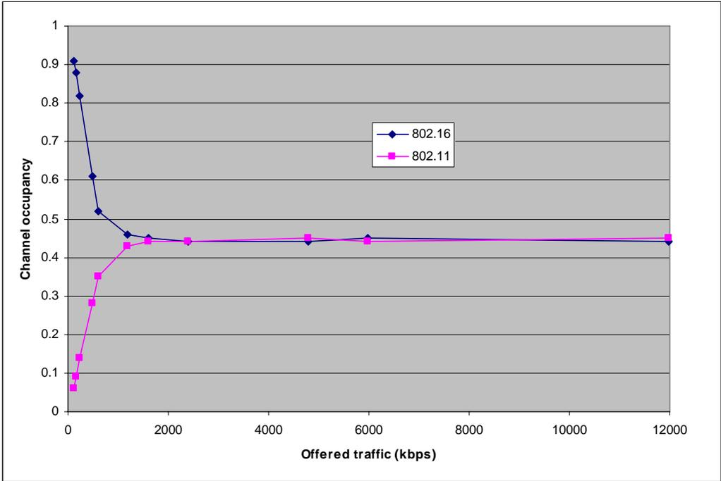
**Figure 12** Collocated simulation configuration – considering fair sharing for 1 802.16 Systems and 1 802.11 System. UtilizationGoal=50%. 46 symbols per frame, downlink=28, uplink=18.
