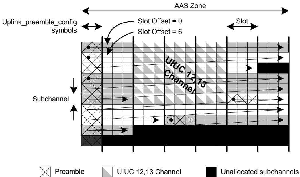
Figure 224b shows a legal UL AAS zone with an UIUC 12,13 allocation that spans all subchannels and is not an integer number of slots in duration.
