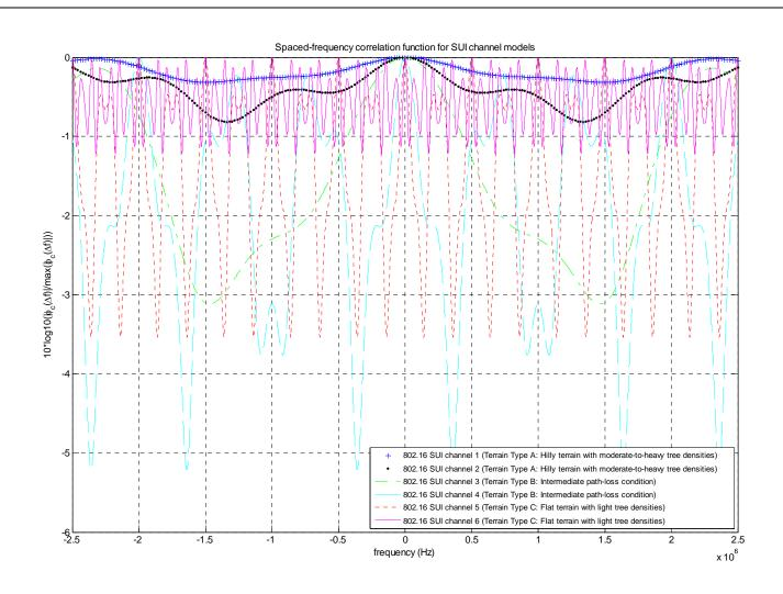
Figure 2. Plot of equation 4 (spaced-frequency correlation) for ITU channel models
