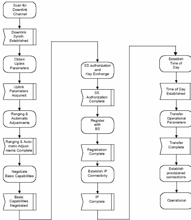
Figure 2. Network entry process for MS (indicated as “SS” in this flowchart).
