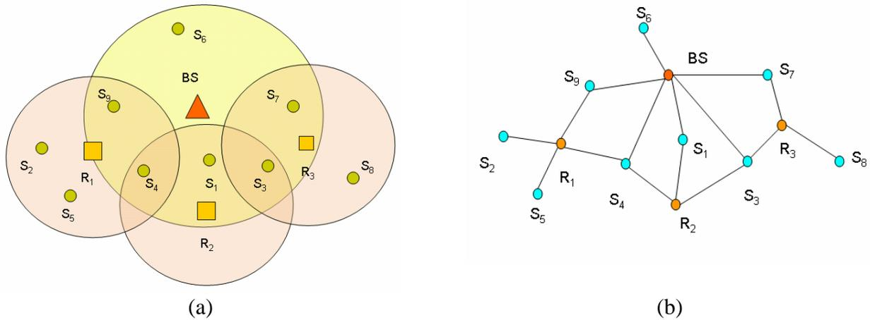
Fig .2. (a) Typical IEEE 802.16 relay network (b) Graph representation of the interference matrix
