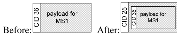
15 16 Figure 12: Before: Packet with CID 36 is routed to Node L. After: Packet with CID 25 is routed to Node 17 E. Node E strips out inner MPDU, and retransmits a packet with CID 36. 18
