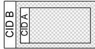
4 5 Figure 10: An inner MPDU with header CID A is encapsulated with an outer MPDU with header CID B. 6
