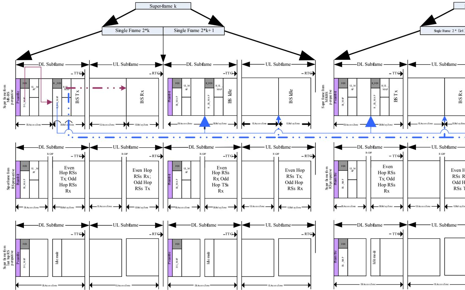
Fig. 1 Dynamic Super Frame Structure.
