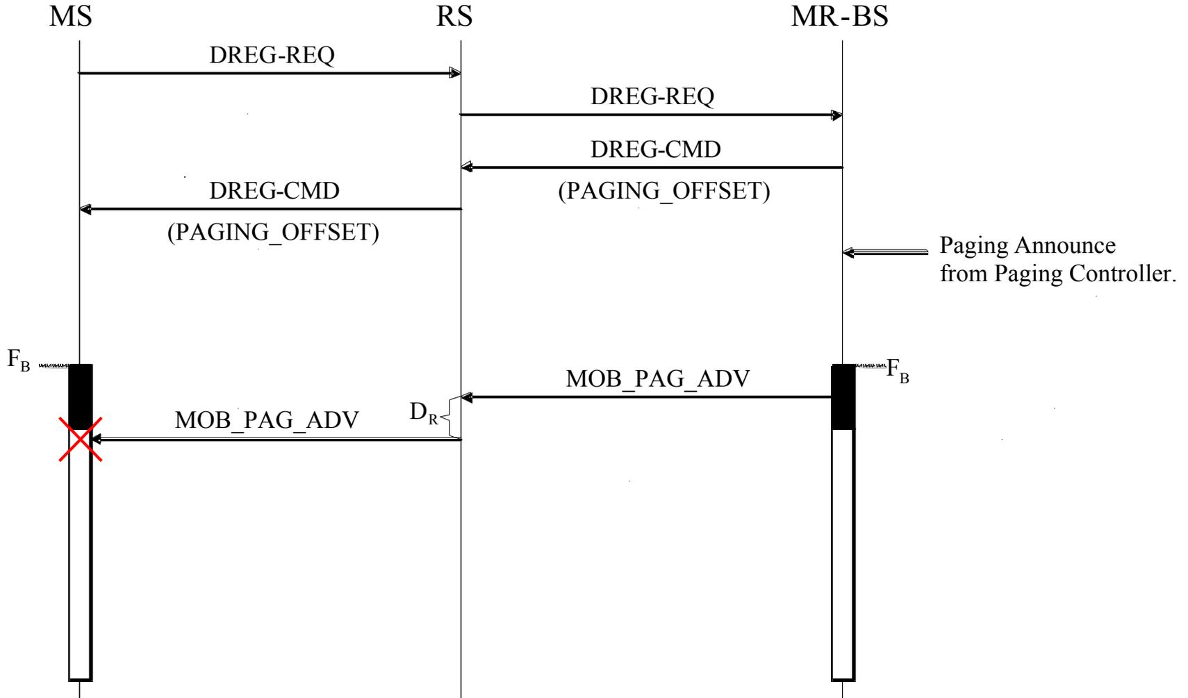
$D_R$  : Relay processing delay of RS
