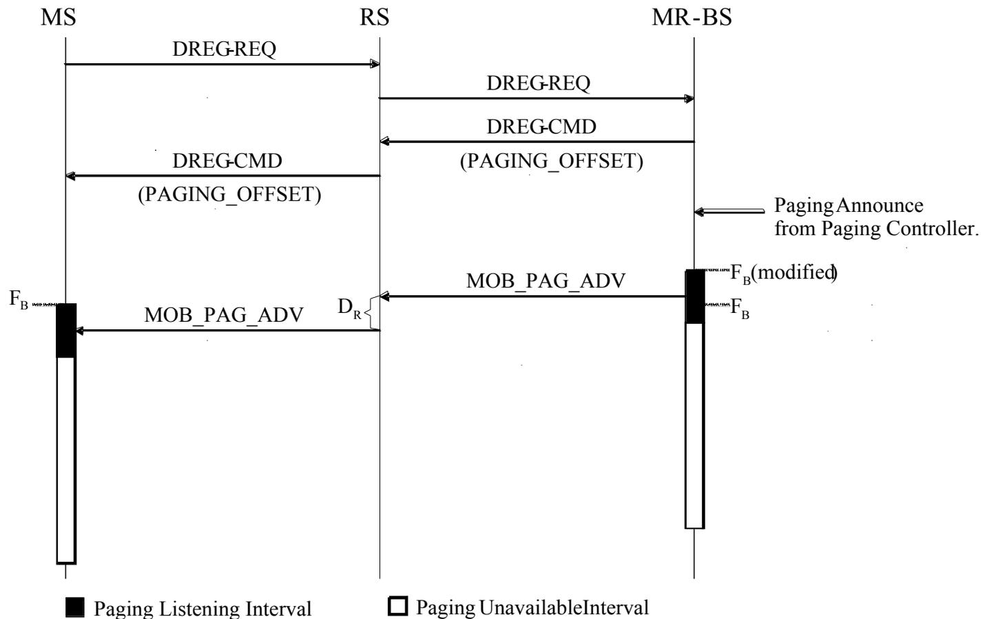
$D_R$  : Relay processing delay of RS
