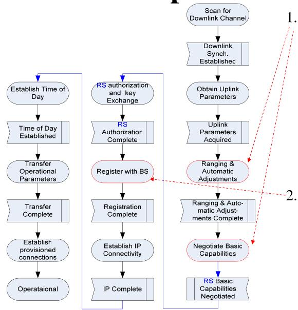
The phases of "Ranging & Automatic Adjustment" and "Negotiate Basic Capabilities" should be modified for various RS modes
