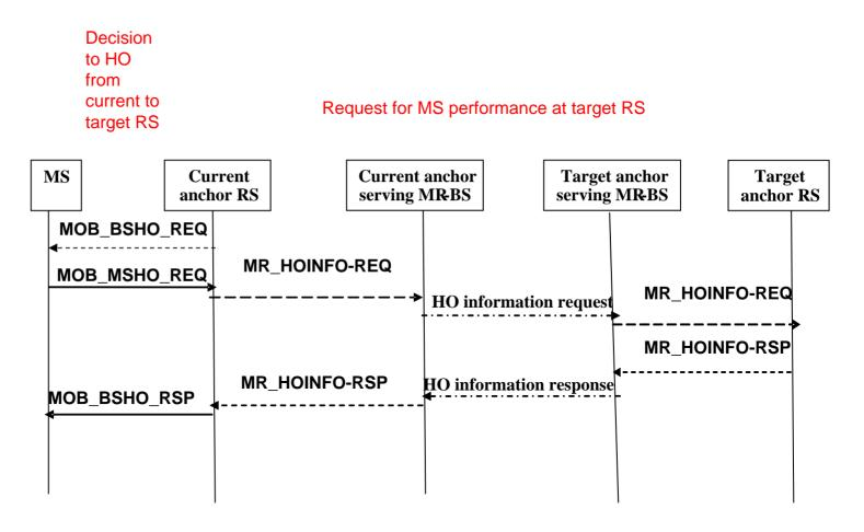
Provide MS performance at target RS to current anchor RS
