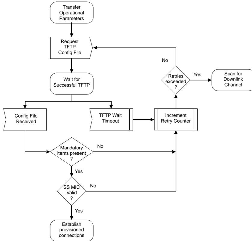
**Figure 1—Transfer Operational Parameters**
