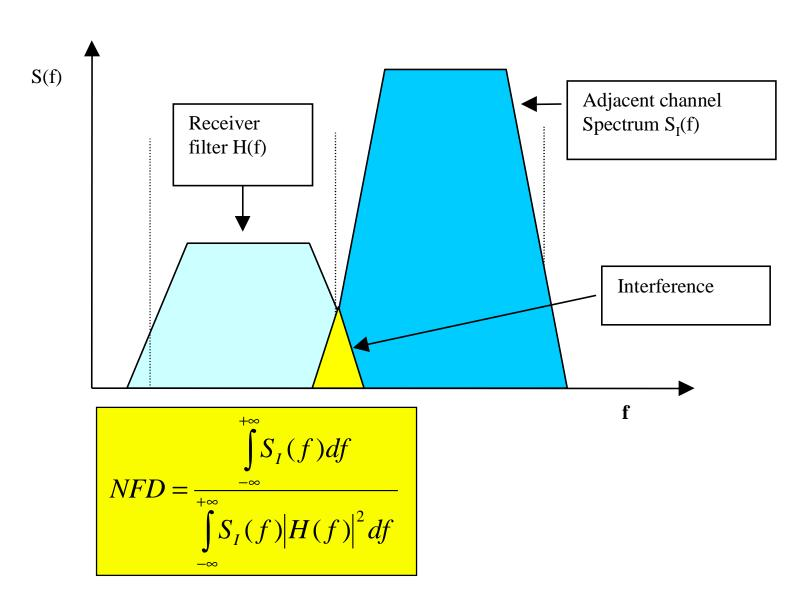
Ratio between the power transmitted by the interfering system and the portion that can be measured after the receiver filter in the adjacent channel
