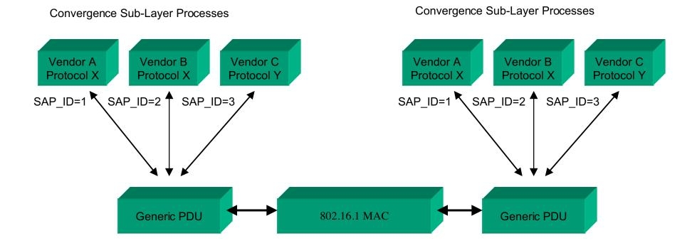
SAP ID is used by the generic SAP to deliver generic PDUs to the appropriate sub-layer process
