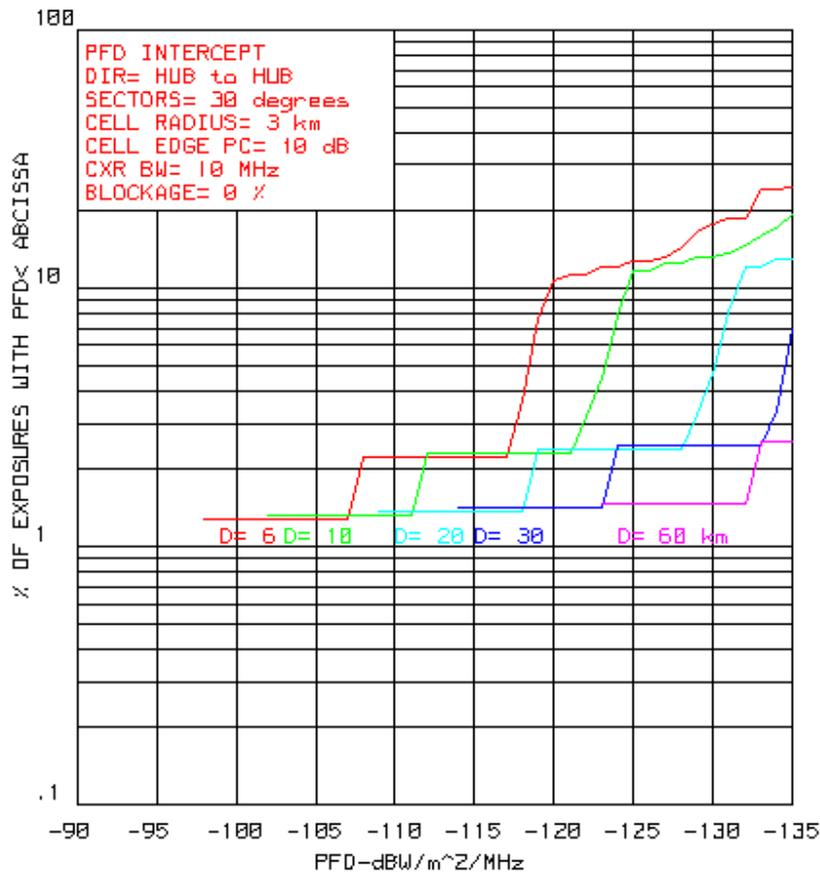
Figure 2. Hub to Hub Interference Probability for 30 Degree TDD Sectors
