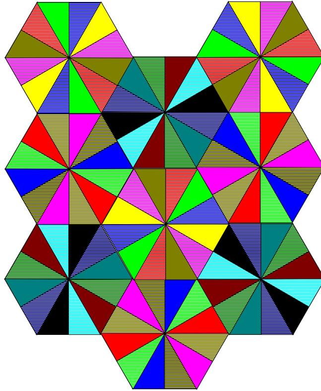
Figure 4 N=9 Frequency Re-Use Cluster for 30 Degree Sectors
