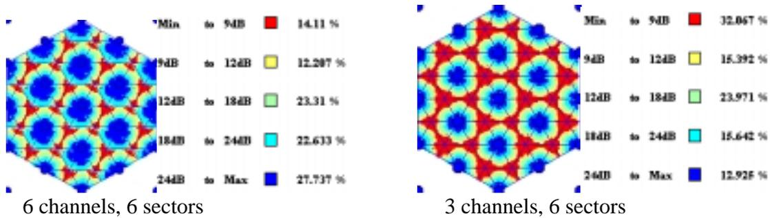
In conclusion, the 6 channels spectrum allocation for a Broadband Mobile System will permit to achieve optimum spectrum efficiency, at high average cell capacity.
