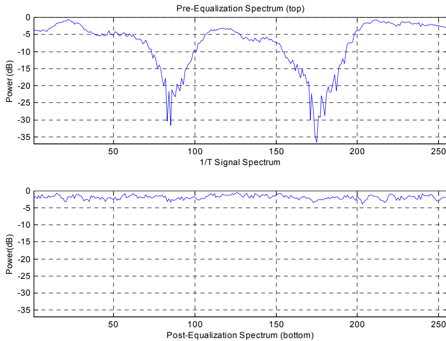
Figure 2-5. Power spectra of pre-SBE and post-SBE signals for ETSI Vehicular Test Channel A.
