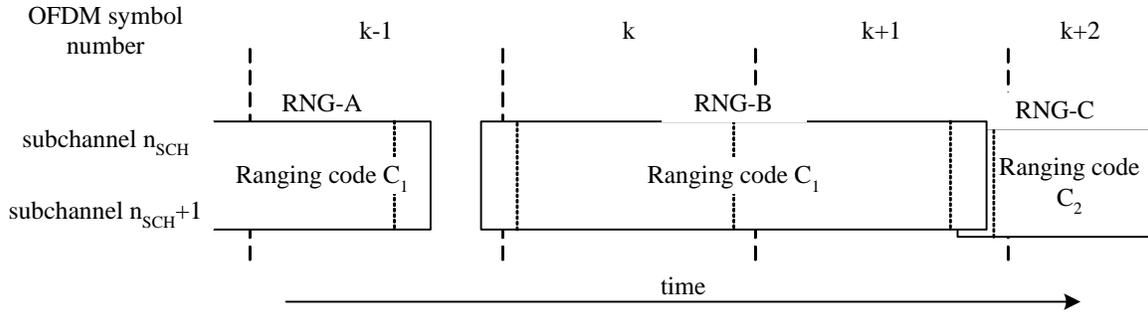
Figure 2–Example of disjoint initial-ranging transmissions
