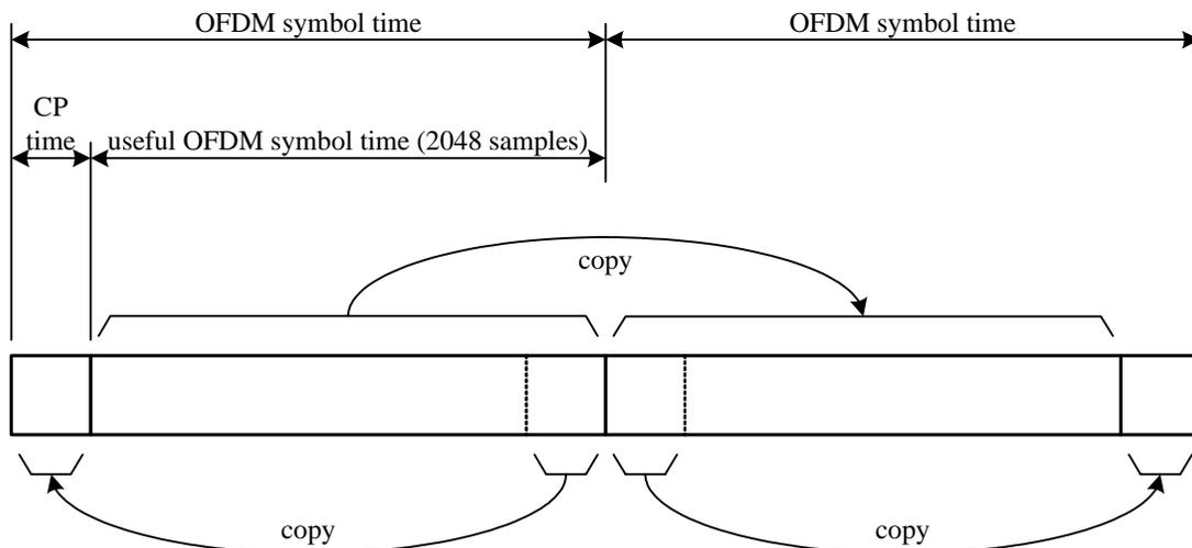
Figure 1–Initial-ranging transmission for IEEE 802.16e OFDMA in the current draft
