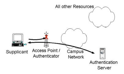
After authentication is successful, the logical "controlled port" becomes enabled – and regular data can then flow across the MAC link.
