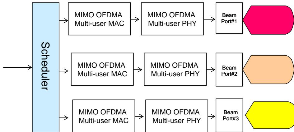
Figure 1 Cell site architecture of the multi-beam MIMO
