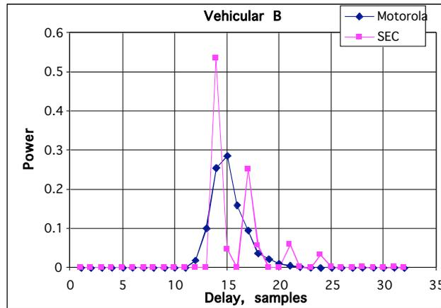
**Figure 6. Typical delay profile. Vehicular B.**
