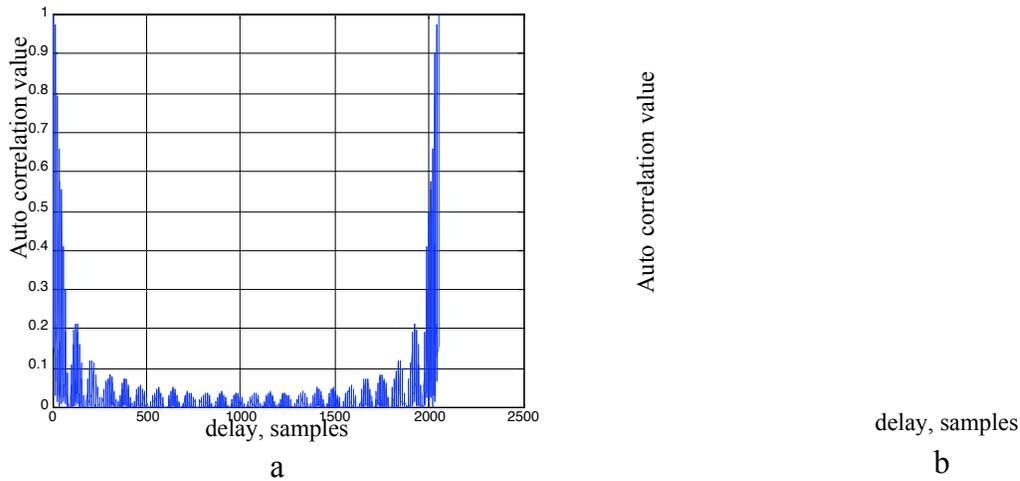
**Figure 3. Scattered subcarriers M-sequence auto correlation properties (a) 2048-fft size, code length 144, contiguous subcarriers GCL sequence auto correlation properties (b) 2048-fft size, code length 144.**
