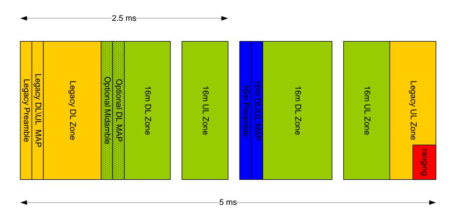
New enhanced preambles and DL/UL MAP are required for 16m users to extend cell coverage.
