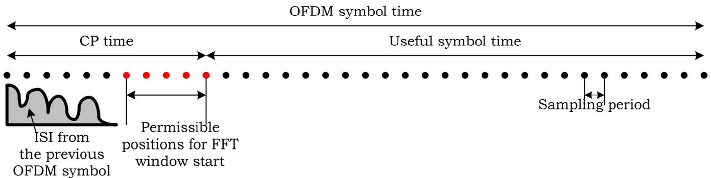
Fig. 1. Permissible positions for FFT window start for data demodulation.
