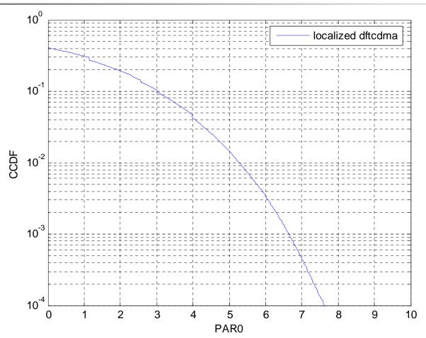
Single DFT precoder with one localized zone exhibits low PAPR as compared to multiple DFT precoders and distributed zones (at the expense of more elaborate receiver algorithms at the BS).
