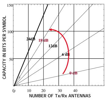
Network MIMO can greatly improve the efficiency of multiple antennas in cellular networks.
