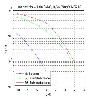
Figure 2 UL control tile: 6x3 vs. 3x6 at 350km/h
