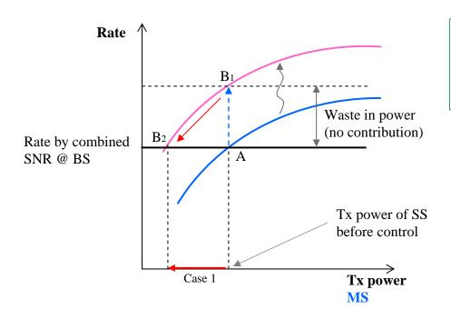
A $\rightarrow$ B<sub>1</sub>: caused by movement (gap exists) B<sub>1</sub> $\rightarrow$ B<sub>2</sub>: gap becomes zero (control is preferred)
