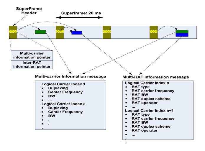
Figure xx Multi-carrier and Multi-RAT information transmission mechanism.
