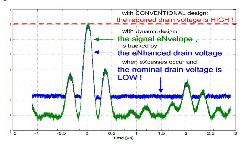
By partial envelope tracking we can change the VCC to the PA and raise It when the signal's peaks occur (Green line: signal envelope) to enable them to be transmitted linearly (Blue Line).
