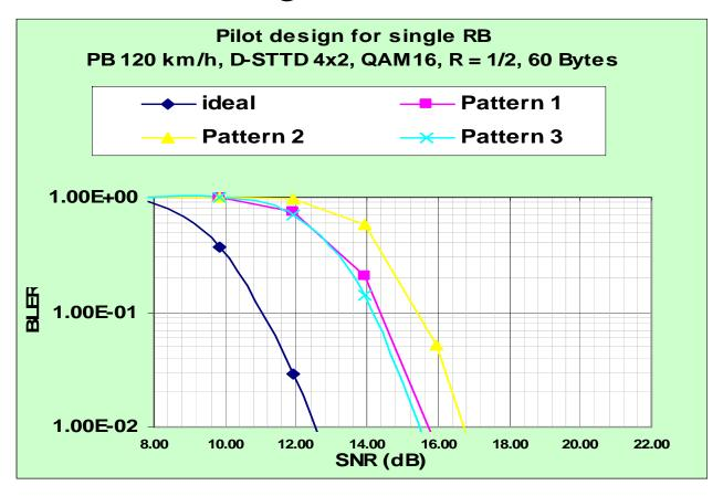
Pattern 3 outperforms patterns 1 and 2 at PB 120km/h
