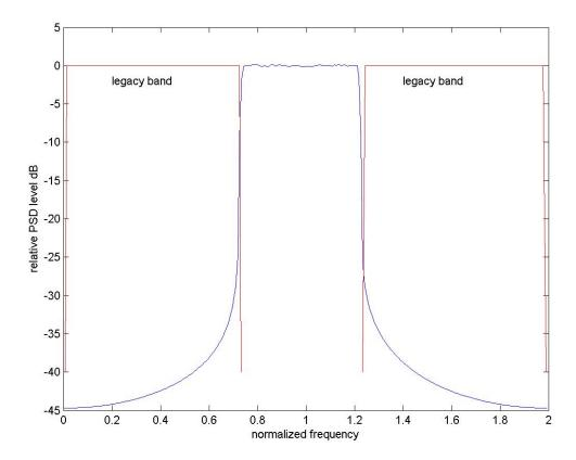
To achieve an acceptable level of interference, the newly inserted OFDM symbol has to be filtered. To apply such filters it has to be employed with guard bands. The guard bands are needed to avoid the need for using sharp filters. Sharp filters tend to prolong the channel impulse response, creating an ISI problem. Filters also will add complexity and power consumption in the transmitter chain.
