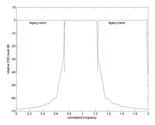
The above figure shows that a drastic reduction in the filter order and/or the guard band can be achieved. This will have a noticeable impact on the complexity of the transmitter and the data rate due to the loss of frequency bins in the guard band.
