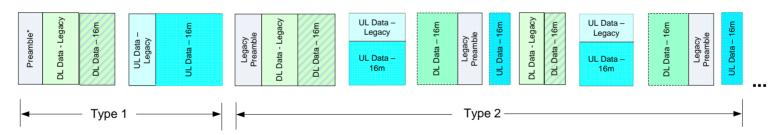
\*Note: Preamble may consists of a Superframe header, legacy preamble sequence, legacy frame configuration and resource control information
