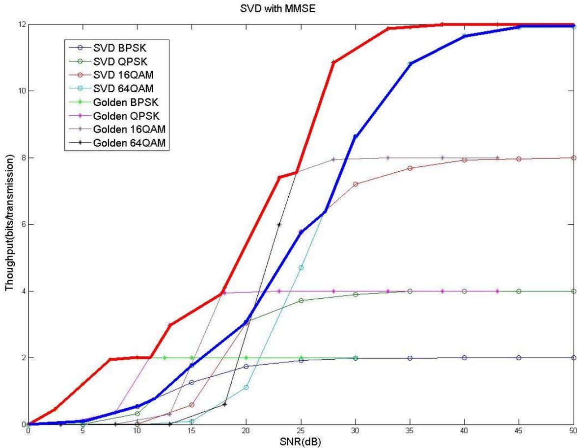
Figure 2: Comparison between Golden STC and SVD with 2-bit transmitter beam-forming matrix feedback.
