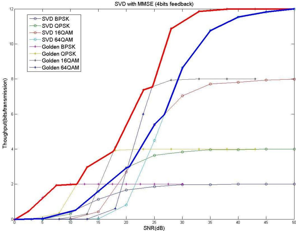
Figure 3: Comparison between Golden STC and SVD with 4-bit transmitter beam-forming matrix feedback.
