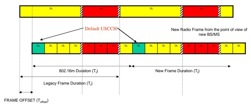
• When operating with legacy support, the default USCCH is located in the first subframe of the 802.16m frame
