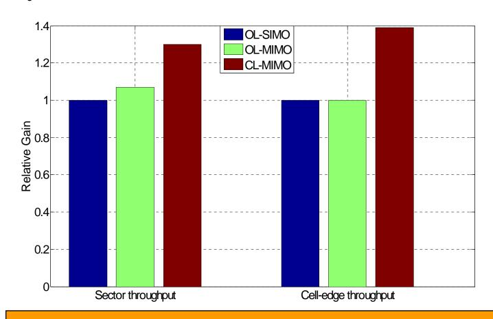
Closed-loop MIMO brings large gain in sector throughput and cell-edge coverage
