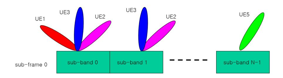
• MU-MIMO is based on *scheduling-directed beamfomring* algorithm
