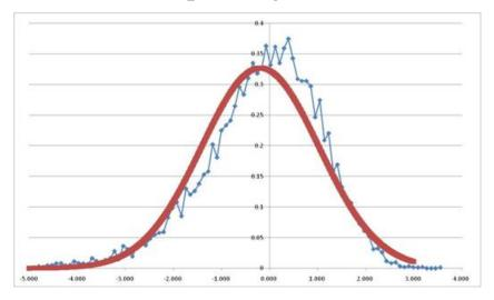
Channel power estimation error can be modeled as Gaussian (0,1.3) in dB scale
