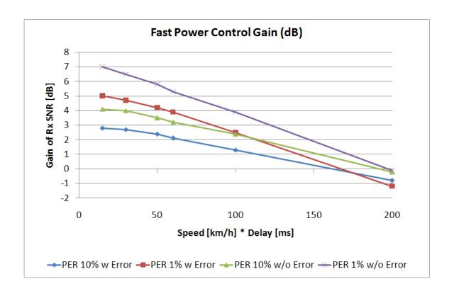
→ As generally known, low speed and short delay between estimation and UL transmission can bring large gain of power control
