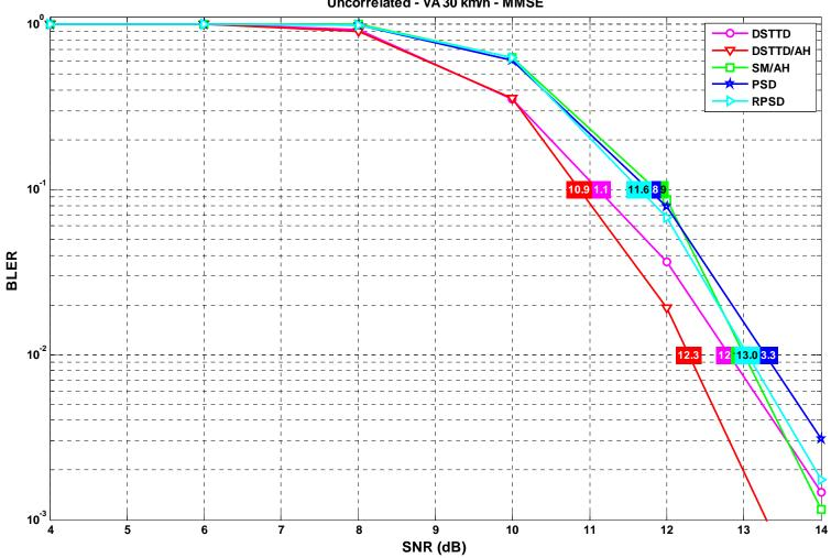
DSTTD/AH has the overall best performance. For reduced receiver complexity, SM/AH is the best candidate compared to PSD and RPSD.
