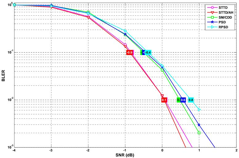
STTD/AH has the overall best performance. PSD and RPSD are inferior to other transmit diversity schemes, and with added complexity due to unitary precoder and phase shift precoder computation.
