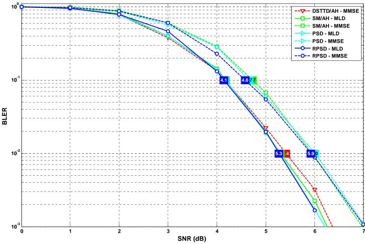
With full MLD receiver, SM/AH, PSD, RPSD have similar performance and are slightly better than DSTTD/AH with MMSE receiver.
