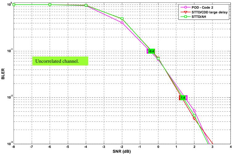
The parameters used for POD and CDD are as suggested in [4]. All three schemes have similar performance. STTD/AH has lower complexity since per RU or per tone phase shift is not needed.
