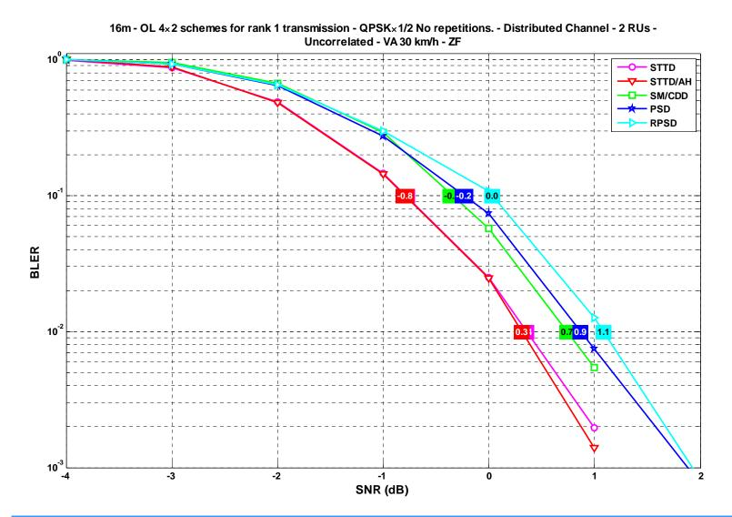
STTD/AH has the overall best performance. PSD and RPSD are inferior to other transmit diversity schemes, and with added complexity due to unitary precoder and phase shift precoder computation.
