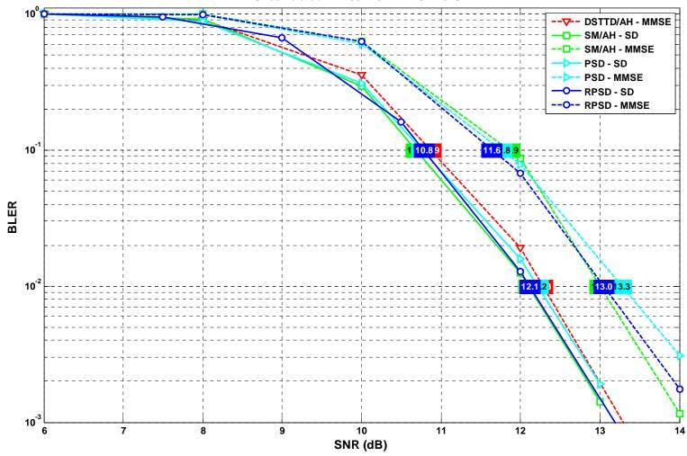
With sphere decoder receiver, SM/AH and RPSD have similar performance and are slightly better than PSD and slightly better than DSTTD/AH with MMSE receiver.
