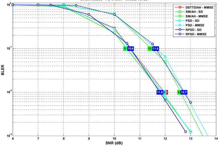
With sphere decoder receiver, SM/AH, PSD and RPSD have similar performance and are slightly better than DSTTD/AH with MMSE receiver.
