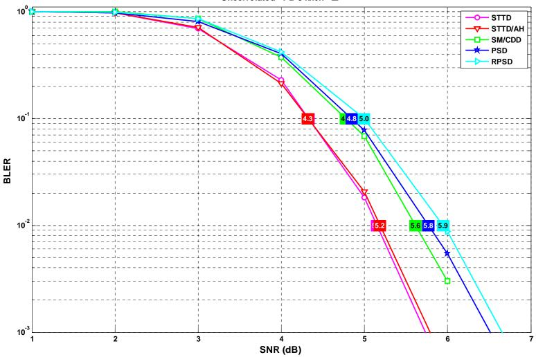
STTD/AH and STTD have the overall best performance. PSD and RPSD are inferior to other transmit diversity schemes, and with added complexity due to unitary precoder and phase shift precoder computation.
