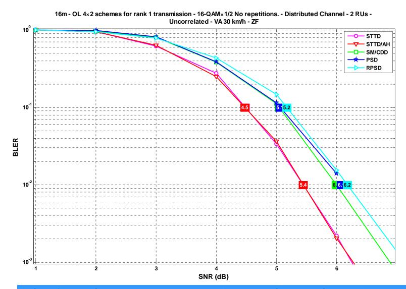
STTD/AH and STTD have the overall best performance. PSD and RPSD are inferior to other transmit diversity schemes, and with added complexity due to unitary precoder and phase shift precoder computation.
