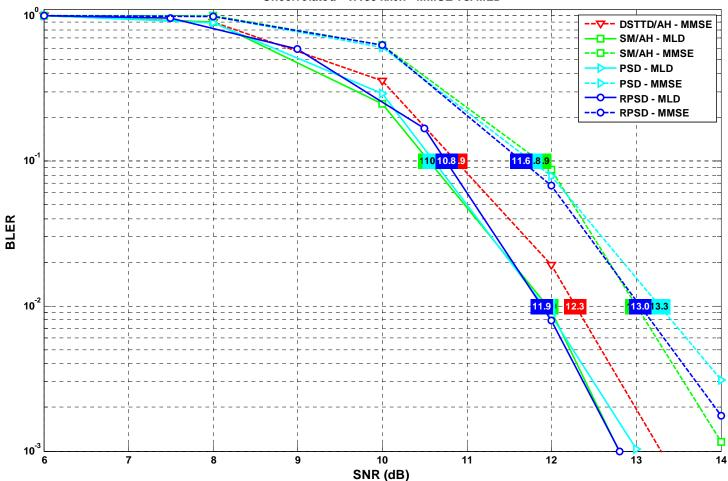
With full MLD receiver, SM/AH, PSD, RPSD have similar performance and are about 0.4dB better than DSTTD/AH with MMSE receiver.
