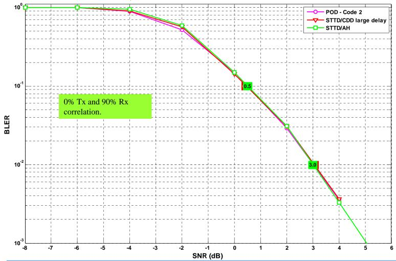
The parameters used for POD and CDD are as suggested in [5]. All three schemes have similar performance. STTD/AH has lower complexity since per RU or per tone phase shift is not needed.
