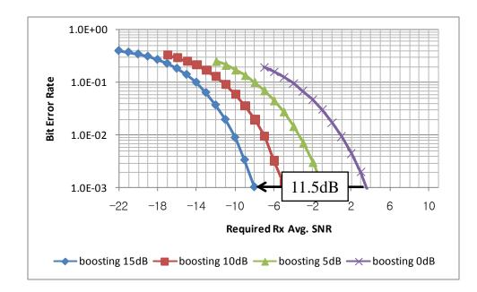
Compared to 0dB boosting, 15dB boosting can obtain only 11dB gain. This is because of channel estimation impairment.
