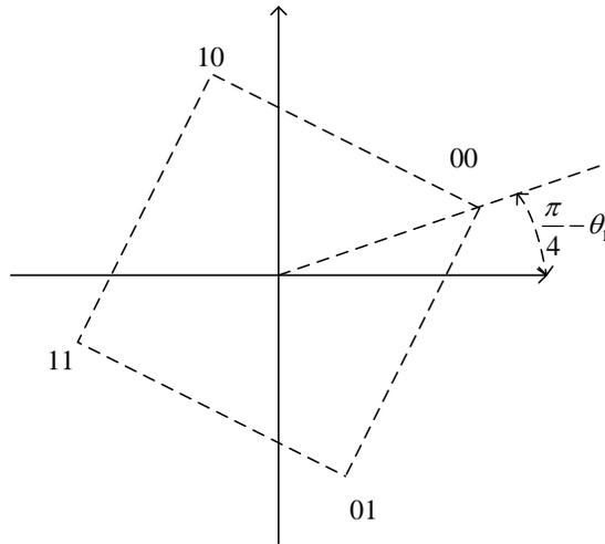
Fig.2 Rotated-QPSK constellation
