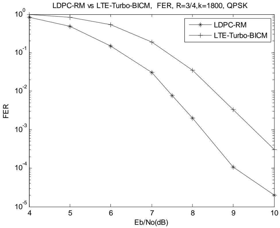
Fig.4 LDPC-RM vs LTE-Turbo-BICM (QPSK, r=3/4)
