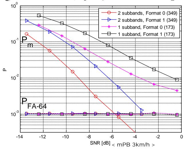
☐ The performance of 2 subbands has 5~6 dB gain compare with that of 1 subband.
