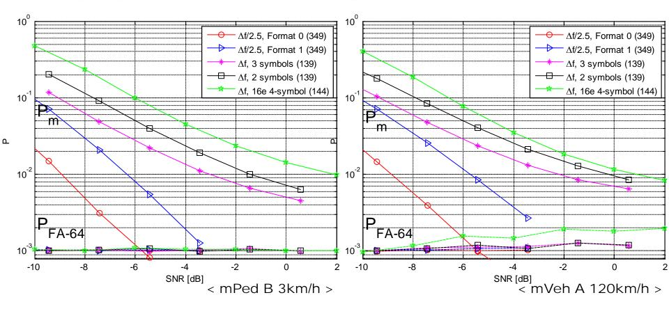
☐ The performance of  $\triangle f/2.5$  subcarrier spacing has 5~6 dB gain compare with that of data subcarrier spacing.
