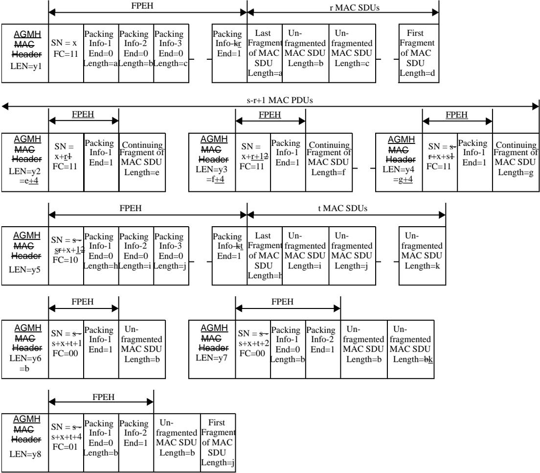
Figure 392—Packing with fragmentation
