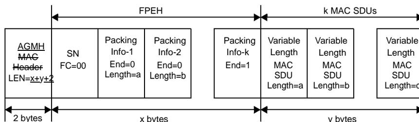
Figure 391— Packing variable length MSDUs into a single MAC PDU
