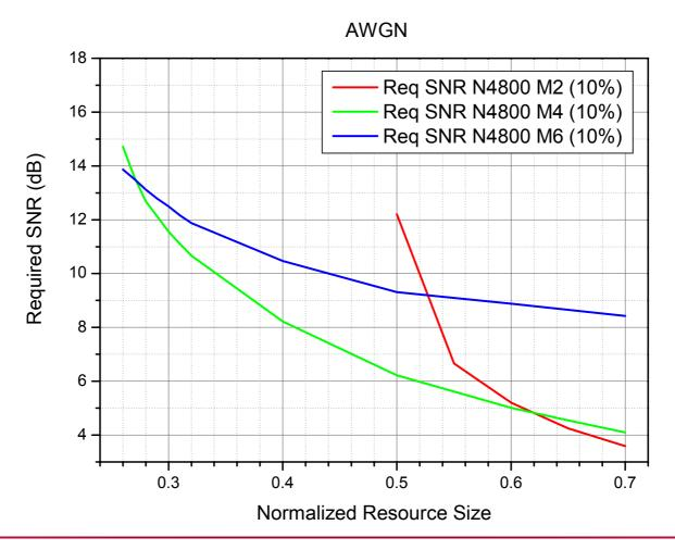
Required SNR (at 10% FER) vs. the modulation order and the Normalized Resource Size (PedB 3km/h)
