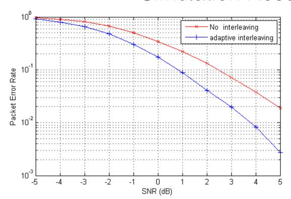
The proposed HARQ scheme adaptive frequency interleaving achieves about **1.3dB gain** over conventional HARQ scheme without frequency interleaving
