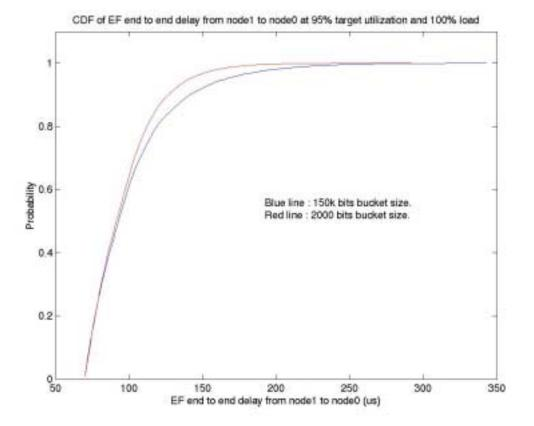
Smaller bucket size can reduce EF delay
