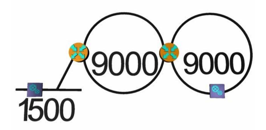
RPR-> Ethernet-> RPR, routed Handled: path MTU discovery
