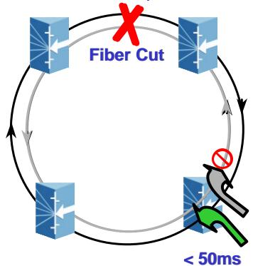
"BLSR like": Only nodes adjacent to a fault know about the fault and wrap packets onto the opposite ring
