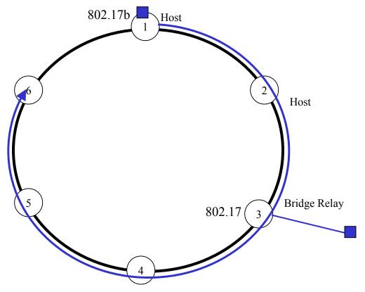
The MAC address method requires these host originated frames to be transmitted using extended frame format.
