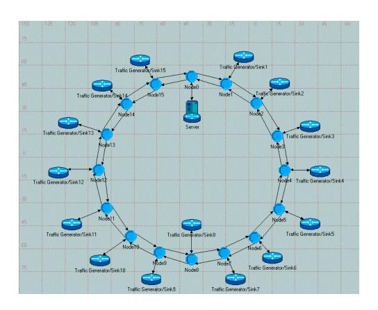
Node 0 is the hub node. Node 1 to Node 15 send traffic to node 0 along counter clock direction (inner ring).
